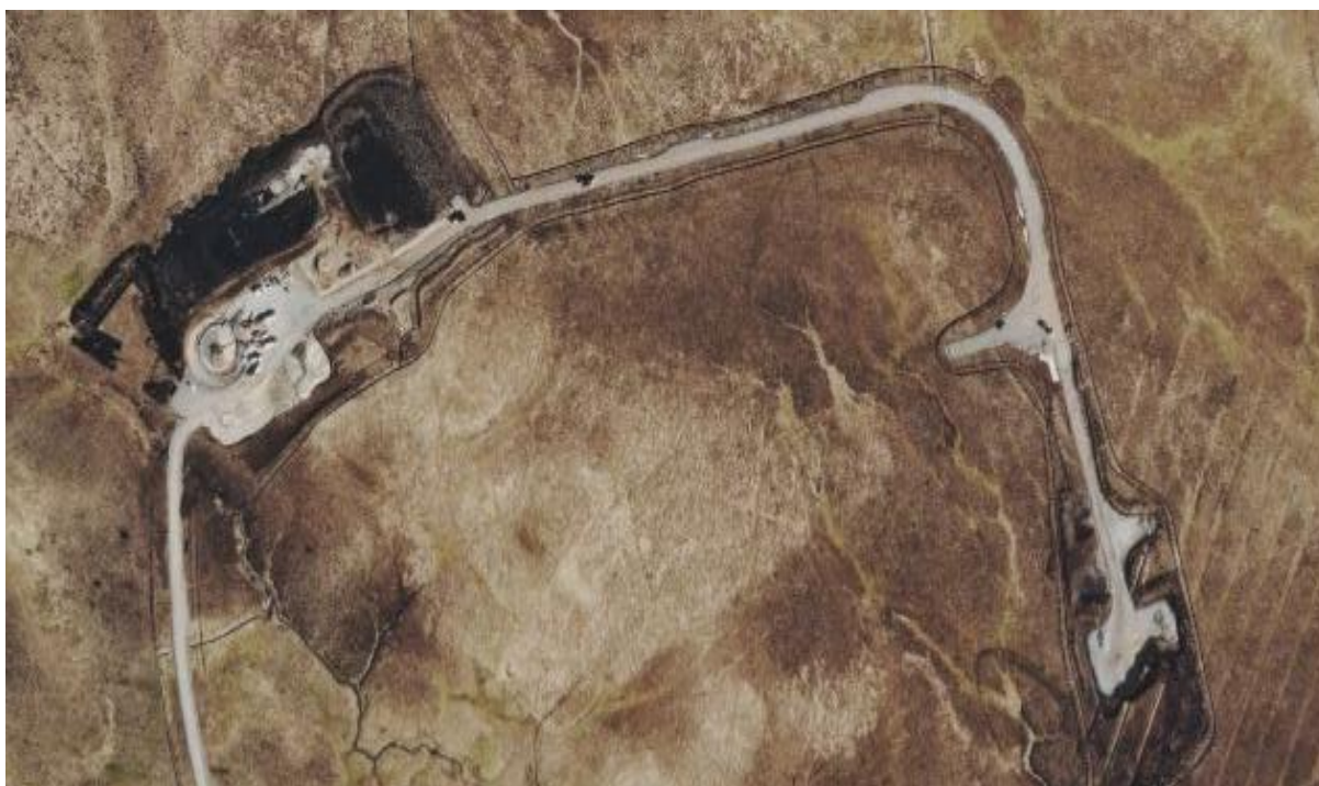
Picture 6: Apple Map aerial imagery (thought to be from winter 2024/2025) showing diggers actively draining and removing peat to build roads and turbine bases as part of a Wind Farm development within the Water of Luce catchment
