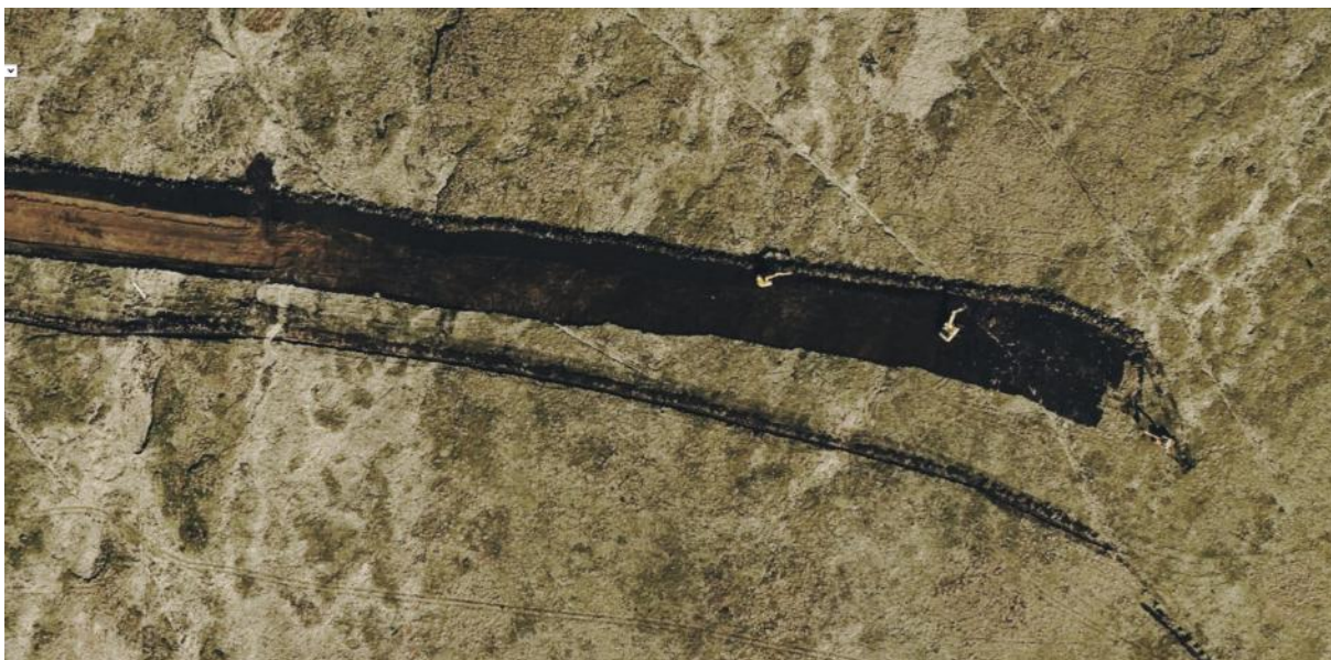
Picture 5: Apple Map aerial imagery (thought to be from summer 2025) showing diggers actively draining and removing peat to build roads as part of a Wind Farm development on the boundary between the Kirkcudbrightshire Dee and Nith catchments
